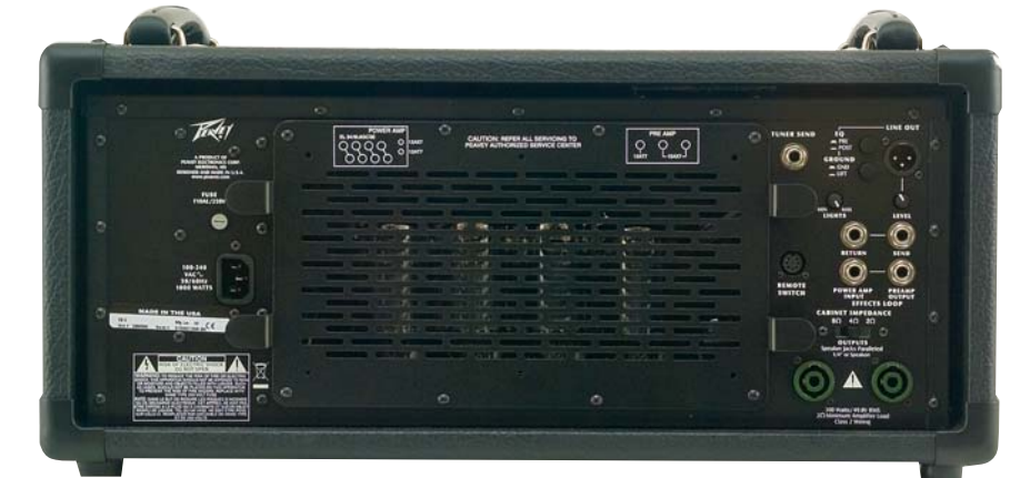
The VB-3's back panel allows easy access to the power tubes for quick replacement.
