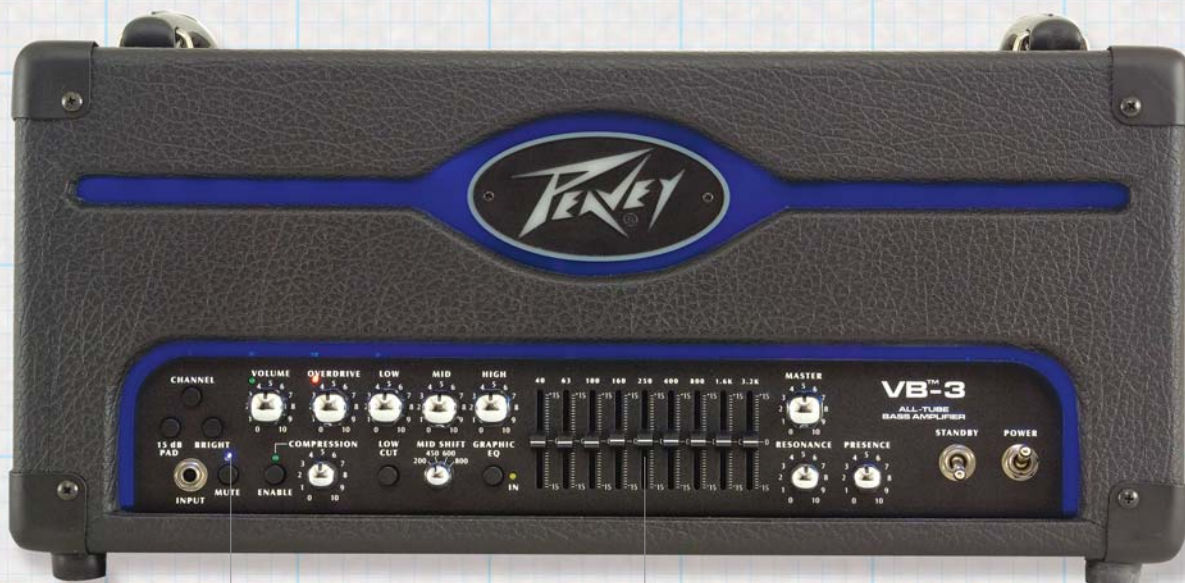
The blue LED above the MUTE switch blinks when the button is depressed.
